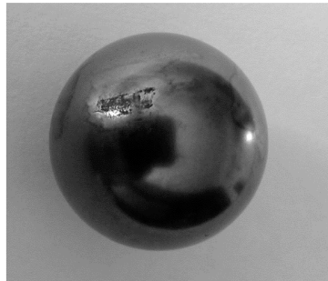
Figure 1. Example of damage to a rolling element of a bearing due to the flow of the bearing current.
