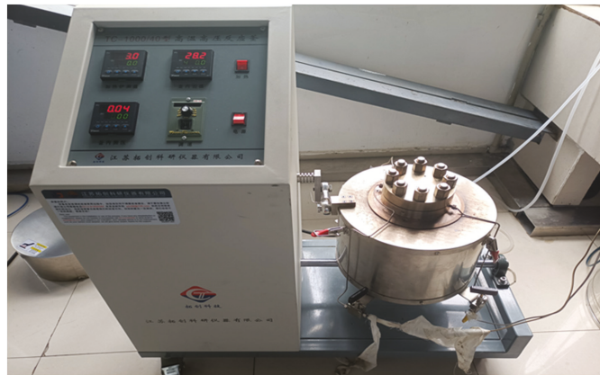
Figure A3. High temperature and high pressure reactor for the generation experiments.
