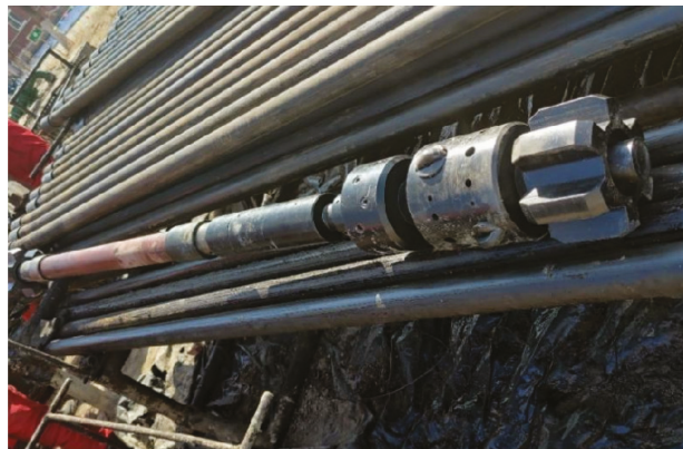
Figure 21. Installation diagram of rotary jet unblock tool.
