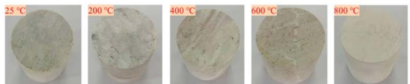
Figure 5. Apparent morphology of marble specimens after high-temperature treatment.
