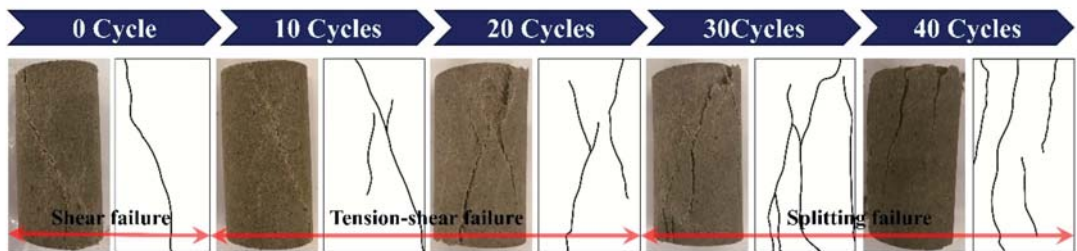
Figure 8. Failure modes of sandstone specimens after undergoing different quantities of F&T weathering cycles in uniaxial compression tests.
