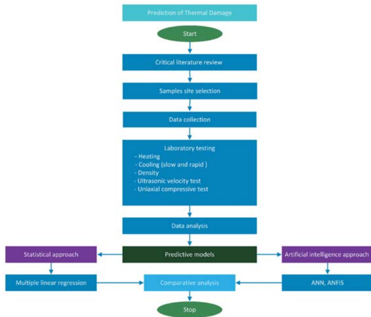
Figure 2. Flowchart of the methodology for the prediction of thermal damage.
