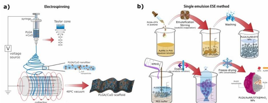
**Figure 3.** Illustration of (a) the electrospinning process and (b) the single emulsion ESE method as well as the further coating of the particles.
