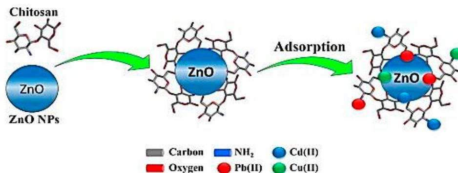
**Figure 10.** Schematic representation of metal ion adsorption by nanocomposite (Taken from [114]).
