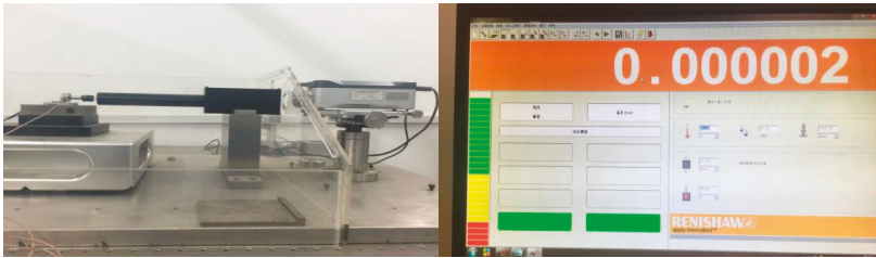
Figure 5. XL-80 laser interferometer ((Renishaw plc, Gloucestershire, UK)).
