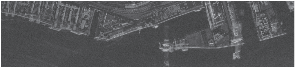
Figure 3. One of the SLC stripes after preprocessed and cropped to the boundaries of the testing set labels. These will be further cropped into non-overlapping tiles and later used as our validation dataset.
