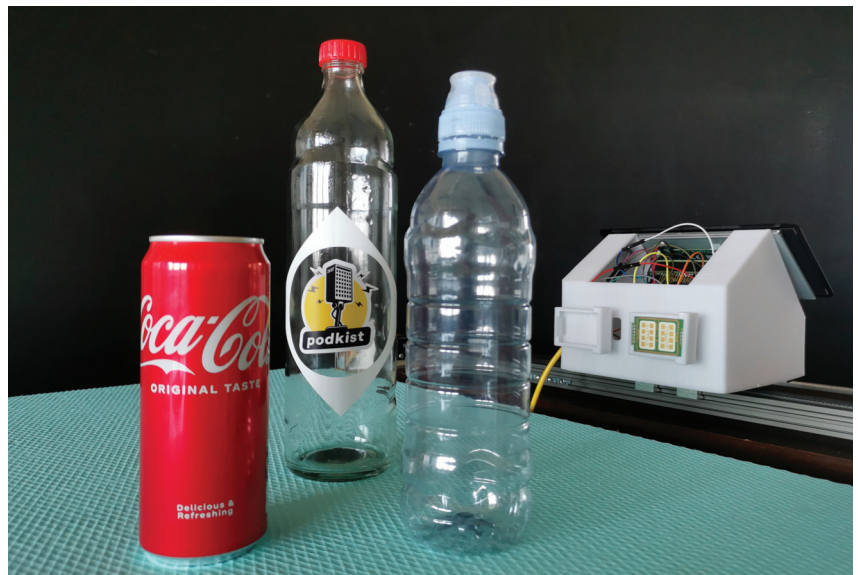
Figure 4. RealSAR objects: aluminium, glass and plastic bottle, and GBSAR-Pi.
