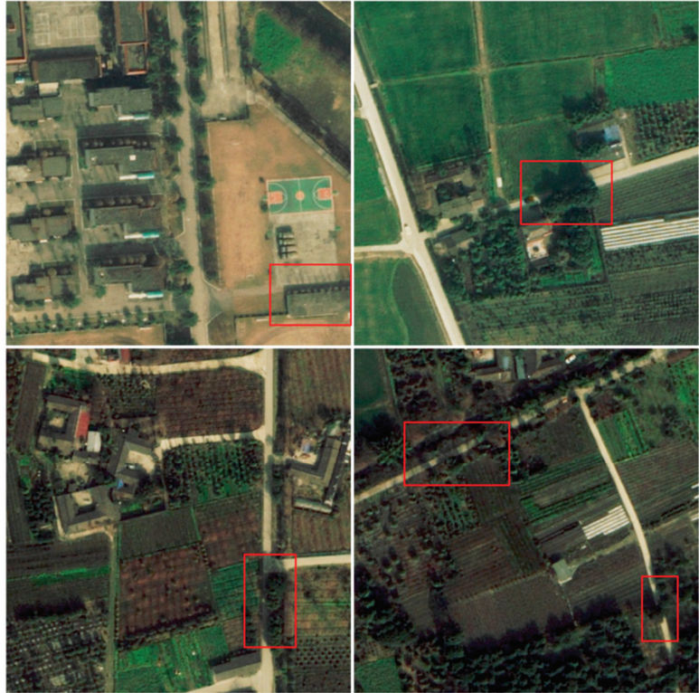
Figure 8. Figures of blocked roads.
