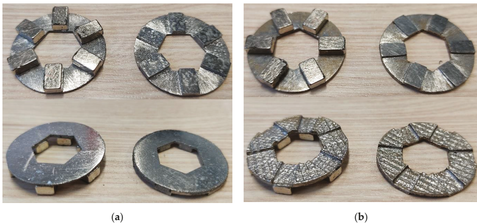
Figure 11. (a) Prototype of the initial design of the coupling; (b) prototype of the optimized design on the coupling.
