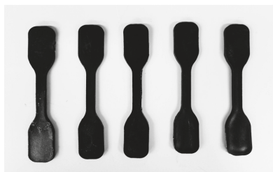
Figure 2. 30 wt. % PP-lignin ASTM D638 Type IV tensile test coupons.
