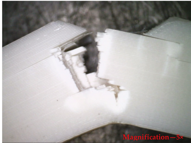
Figure 18. Optical microscopic view of the deformed specimen after impact test, side view.
