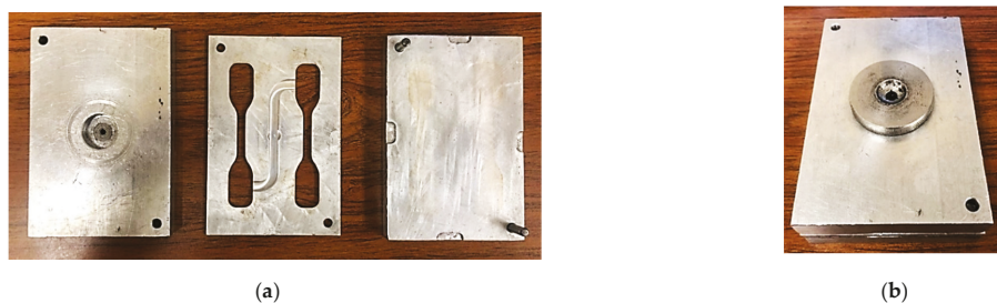
Figure 1. Three-piece injection mold designed for lignin blends: (a) showing the three separate pieces; (b) assembled mold with the sprue.
