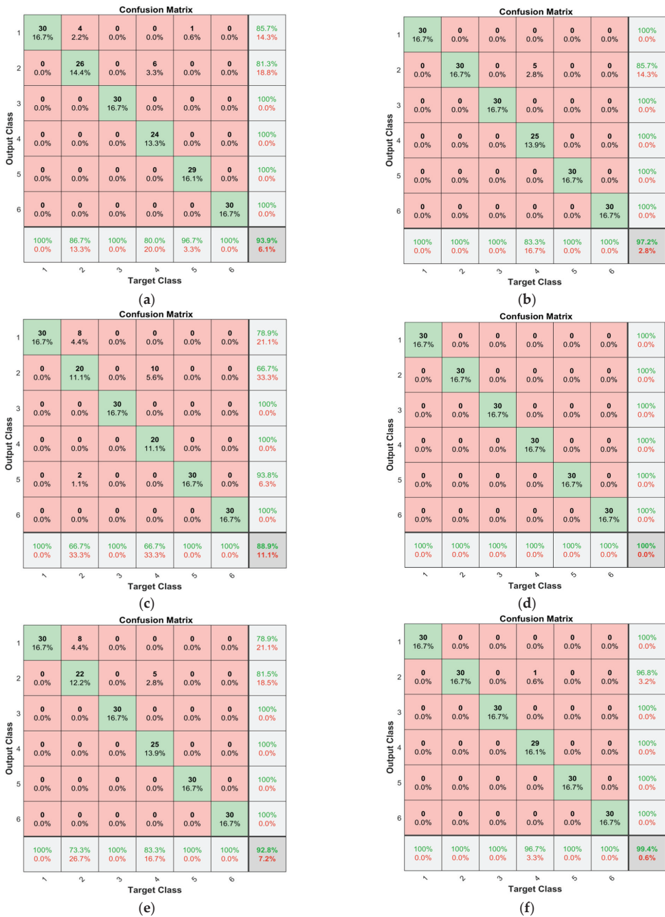
Figure 13. Confusion matrix of diagnosis results of different models based on dataset A and B. The following are the results of: (a) 1-DCNN from dataset A; (b) 1-DCNN from dataset B; (c) 1-DDCNN from dataset A; (d) 1-DDCNN from dataset B; (e) 1-DDCNN II from dataset A; (f) 1-DDCNN II from dataset B.
