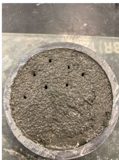
Figure 2. Gap generated in paste indicating the start of setting time.
