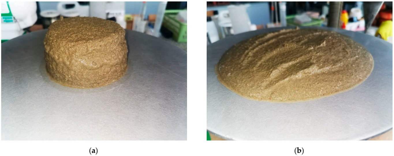
Figure 1. (a) View of the C0 sample after removing the form for flow research; (b) View of the C0 sample after flow test.
