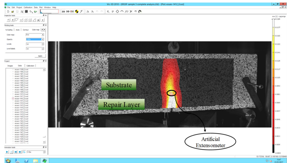
Figure 9. Placement of an artificial extensometer at the interface.
