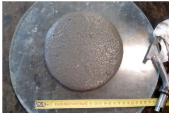
Figure 4. Measurement of the stabilized biscuit.
