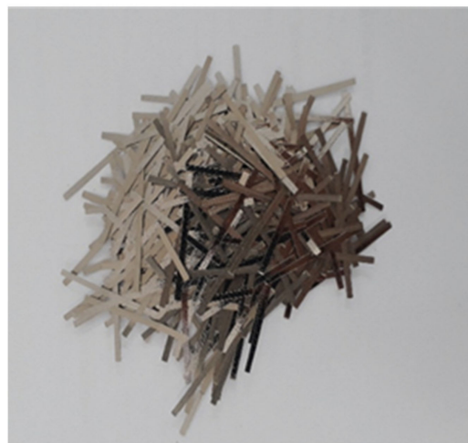
Figure 2. 30 mm-long metallic fibres.
