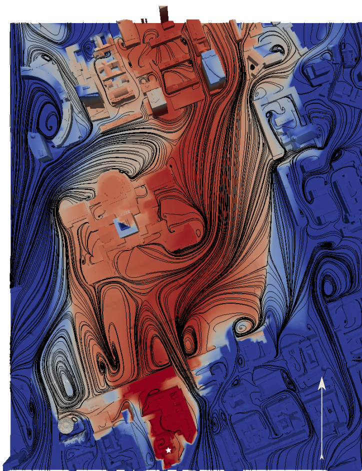
Figure 2. Visualisation of the ground concentration of a pollutant on a logarithmic scale that was released on a roof top (white star), which is in the bottom part of the figure. The complex wind field is visualised using streamlines, and the inflow wind direction is given by the white arrow. The geometry is that of the Parade Square in Warsaw, Poland.
