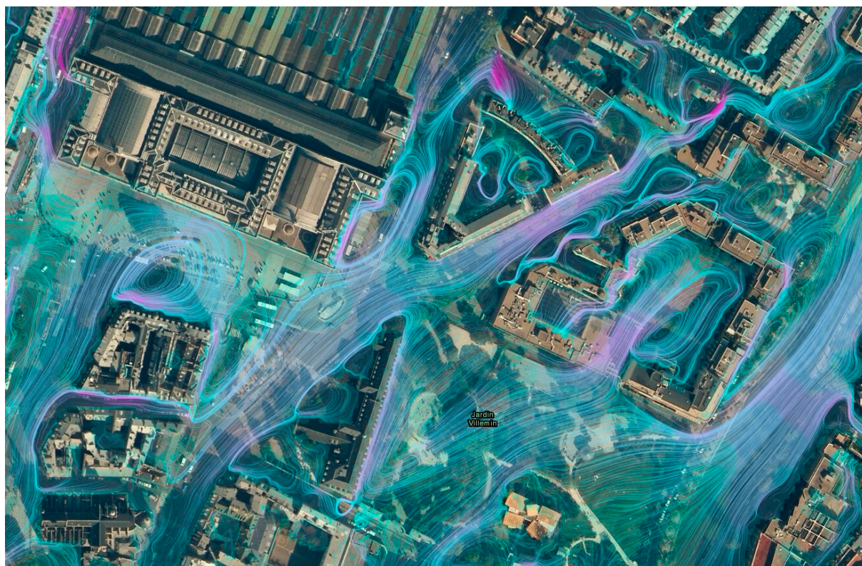
Figure 6. Closeup view of the flow streamlines computed in the streets south and east of the train station. The wind speed ranges from 0 m/s in cyan to 2 m/s in magenta.
