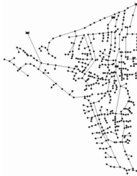
Figure 4. Layout of Balerma network (BIN) [21].
