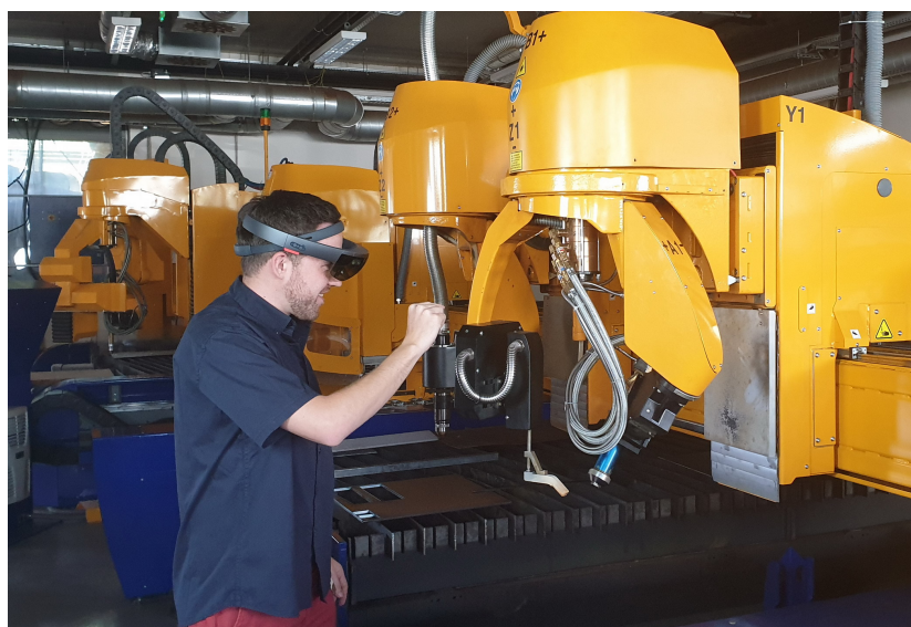
Figure 2. Testing of augmented and mixed reality for cutting machine maintenance.
