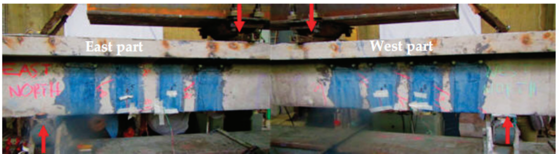
Figure 16. The East and the West parts of the prototype RC T-beam with the 1st shear strengthening scheme under four-point bending.
