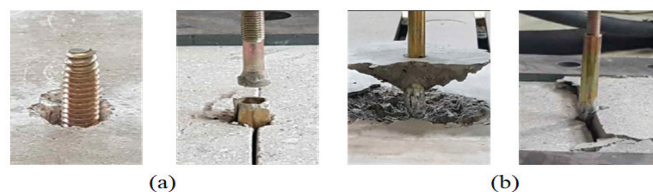
Figure 11. Failure mode for static pull-out tests: (a) M10 set anchor; (b) M12 set anchor.
