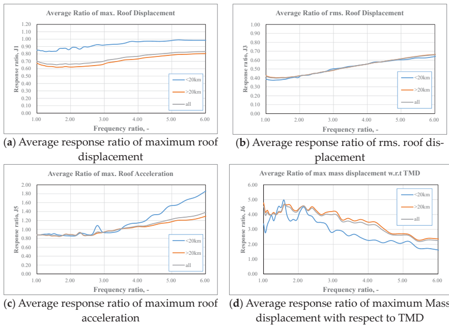
Figure 9. Response ratio of Structure with the ISAMD with W_V:W_A = 1:0 , without auxiliary damper and spring under 26 seismic excitations.
