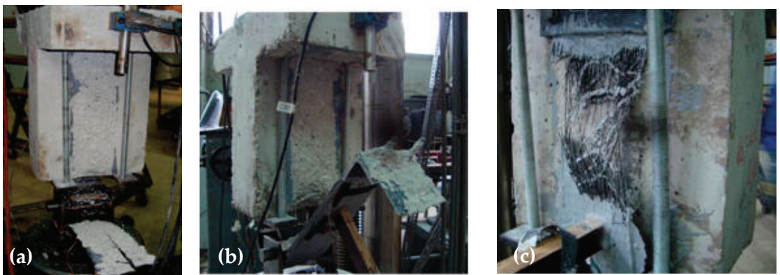
Figure 12. (a) Debonding mode of failure. (b) Failure of the anchoring scheme accompanied with debonding. (c) Tensile failure of the FRP strip.
