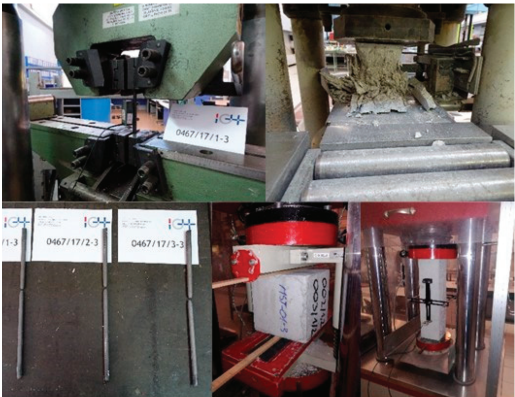
Figure 8. Performance testing of concrete and steel.
