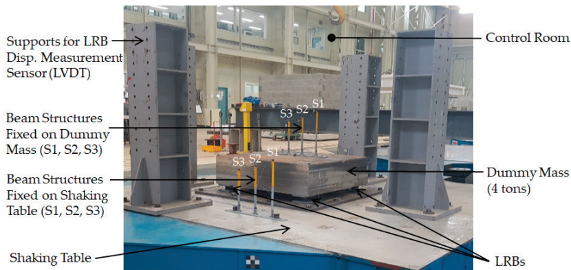
Figure 1. Photos of test mockup with four LRBs and four tons dummy mass system.
