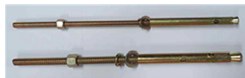
Figure 5. Post-installed anchors applied to experiments.
