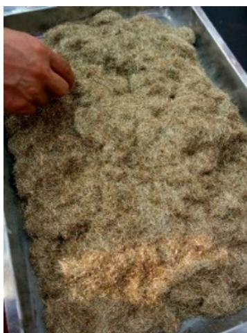
**Figure A1.** Steel fiber in concrete.
