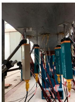
**Figure 4.** The arrangement of the displacement sensor.
