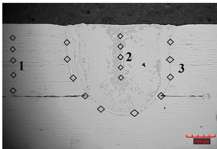
Figure 10. The scheme of microhardness measurements: the tube core material (1); the central part of the penetration (2); near the fusion penetration line (3).
