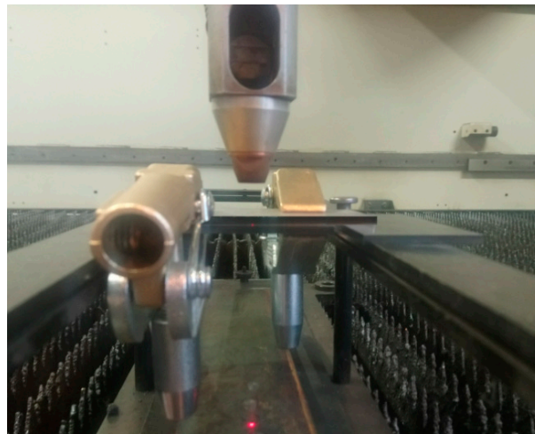
Figure 4. Laser-welding station with lap joint low-carbon steel configuration.
