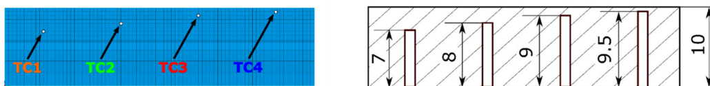
Figure 25. Scheme of thermocouple placement on the cross-section of samples in the axis of welded beads.
