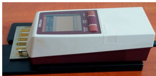
Figure 2. A view of the portable surface roughness tester SJ-210 SurfTest Mitutoyo during measurements of roughness on the surface of stringer beads produced by laser gas nitriding of titanium alloy Ti6Al4V.
