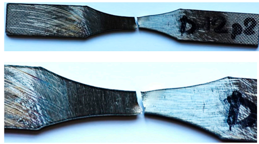
Figure 10. The hourglass specimen made of the Docol 1200 M steel with the micro-jet cooling weld after fatigue test at maximum value of stress of 500 MPa.
