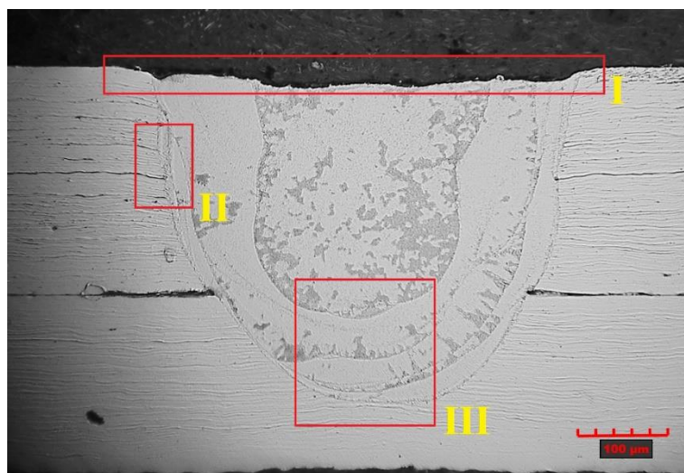
Figure 6. Structure of the weld with the characteristic areas of the joint marked. I – weld face, II and III - the fusion penetration line of the weld into the base material.
