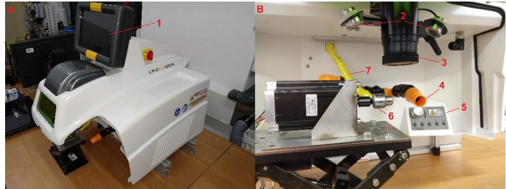
Figure 3. View of the SISMA LM-D210 laser bench. (A)—general view, (B)—workspace view. 1—front touch panel, 2—lighting spots, 3—laser head, 4—gas extractor, 5—manual parameter set panel, 6—rotary motor, 7—nozzle of gas shield.
