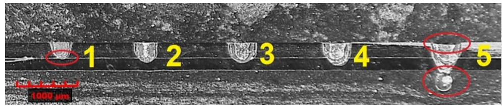
Figure 4. View of obtained welds for lap joints in cross-section.
