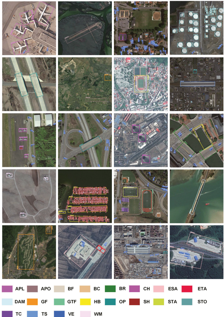
Figure 8. Depictions of the detection results on the DIOR-R dataset test set. We use bounding boxes of different colors to represent different categories.
