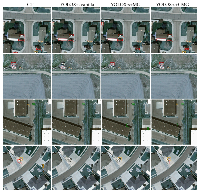
Figure 5. Qualitative results of YOLOX-s on VEDAI25. The contrastive mutual guidance helps to recognize intricate objects. The number and color of each box correspond to one of the classes, i.e., (1) car, (2) truck, (3) pickup, (4) tractor, (5) camper, (6) ship, (7) van, and (8) plane.
