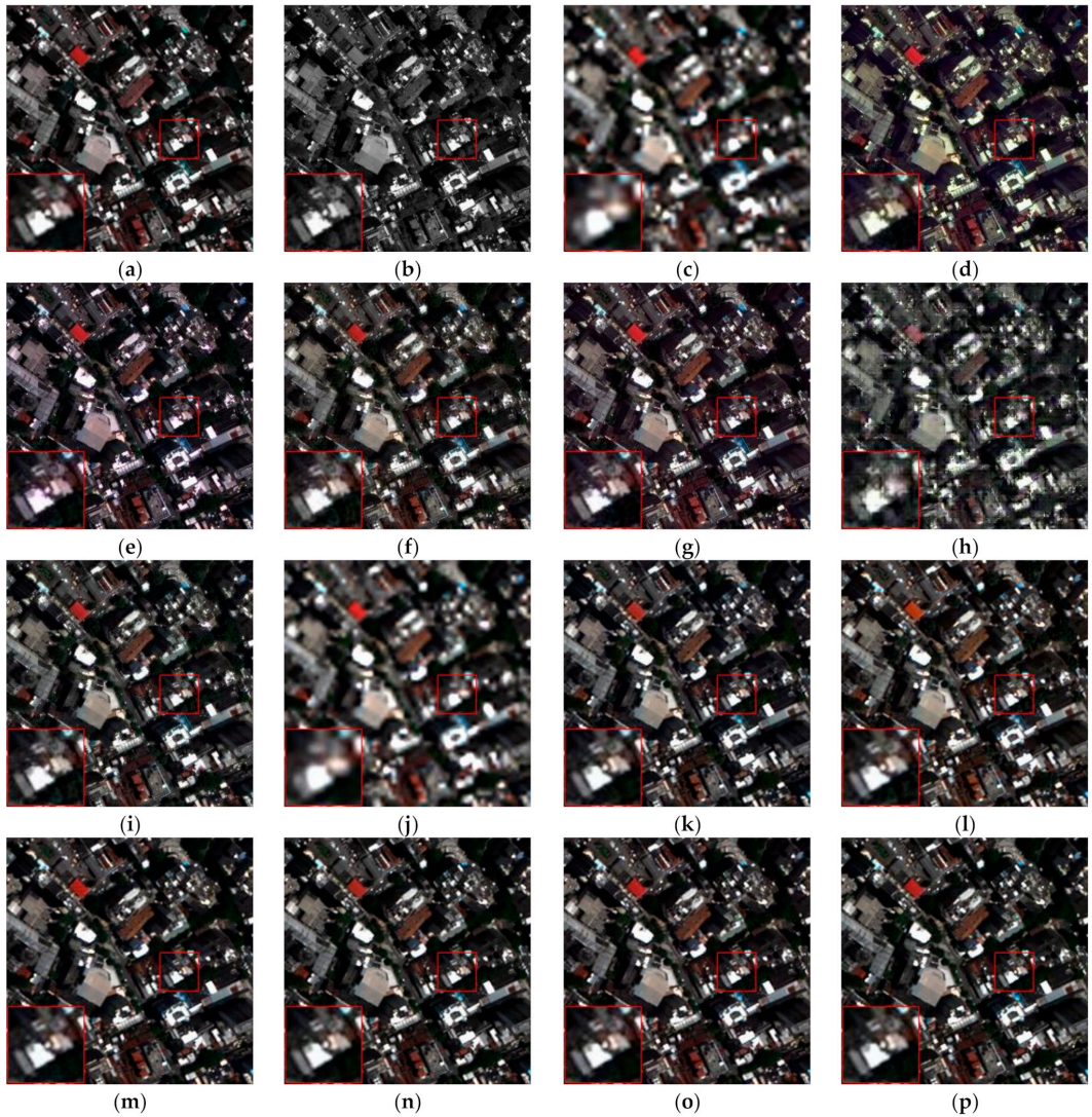
Figure 8. Results using the WorldView-3 dataset with four bands (resolutions of 256 \times 256 pixels): (a) reference image; (b) PAN; (c) LRMS; (d) IHS; (e) PRACS; (f) HPF; (g) GS; (h) DWT; (i) GLP; (j) PPXS; (k) PNN; (l) DRPNN; (m) PanNet; (n) ResTFNet; (o) TPNwFB; (p) ours.
