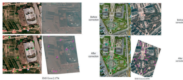
Figure 9. These are the results of selecting evenly distributed points from satellite images and corrected UAV images, and calculating the errors among them.
