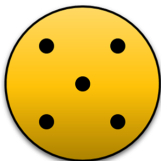
Figure 2. Shore A hardness probing sites along the sample surface.
