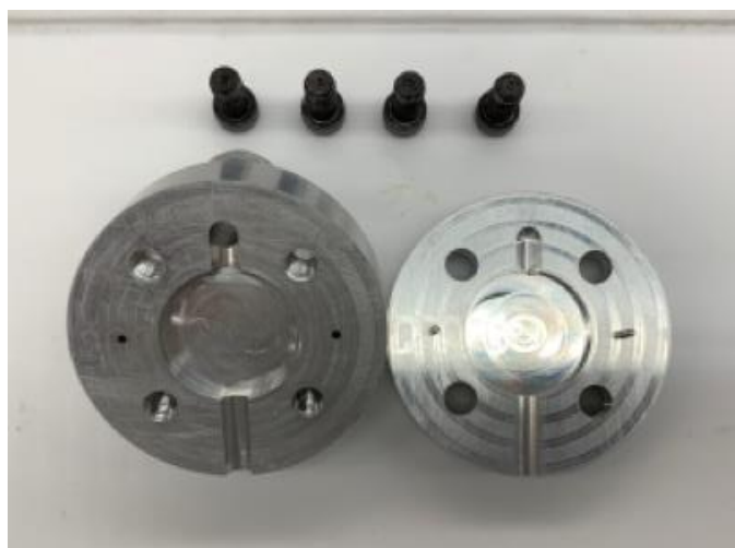
Figure 1. Custom split-die injection mold with a cavity size of 25.4 \times 6.35 mm used to form samples for compression and hardness testing.
