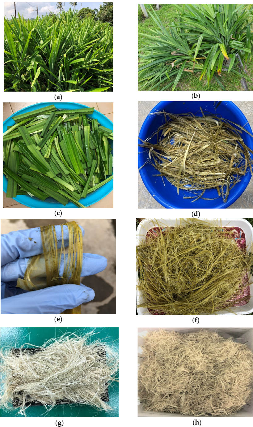
Figure 1. Pictorial view of fibre extraction (a) Pandanus amaryllifolius plant; (b) cut bulk of leaves; (c) leaves cleaned and immersed in the water; (d) after 2 weeks; (e) skin degraded and removal of fibres; (f) extracted fibres collected and dried under sunlight; (g) ungrounded fibres after being further dried in oven; (h) ground (short fibres) PAF.
