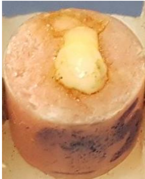
Figure 3. Image of assembly of the natural teeth within the self-cured acrylic resin mold.
