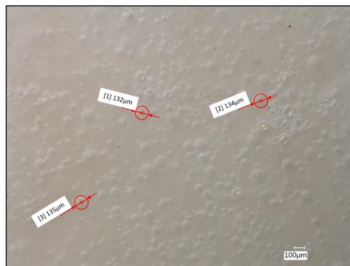
Figure 6. PHB/microsphere (3%) composite sample surface with measured pore diameters of fully formed microspheres. Image taken at 100\times under partial-ring lighting conditions.
