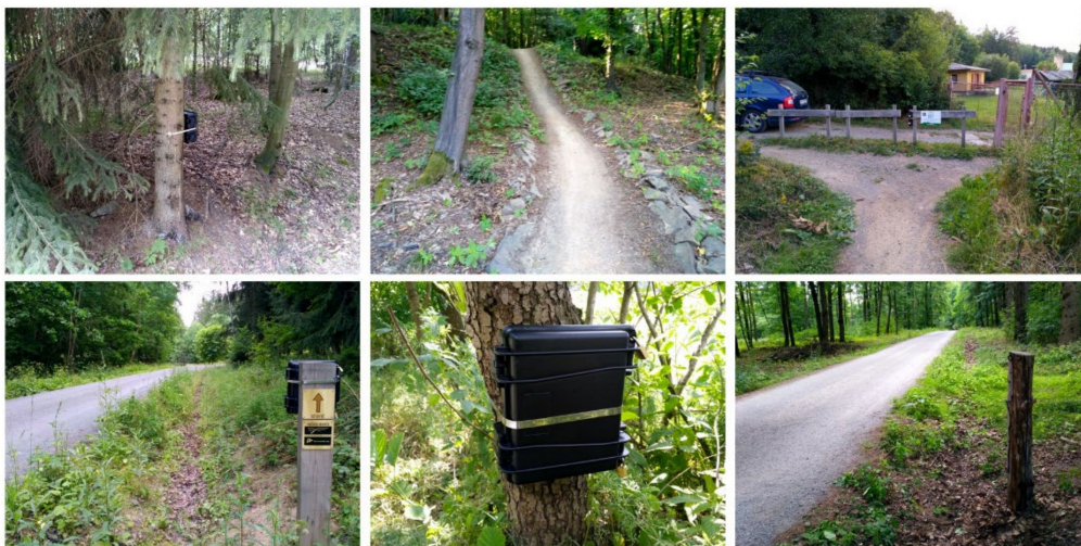
Figure 3. Examples of counter installation.
