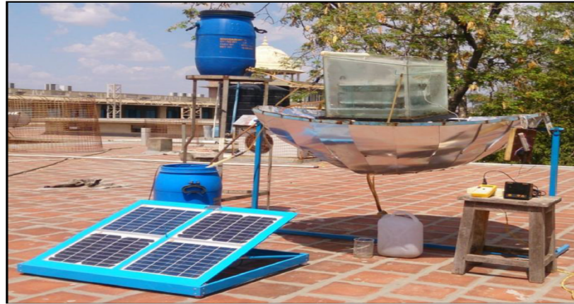
Figure 20. Photograph of a triple basin solar distillation still coupled with an immobile SDC [99].
