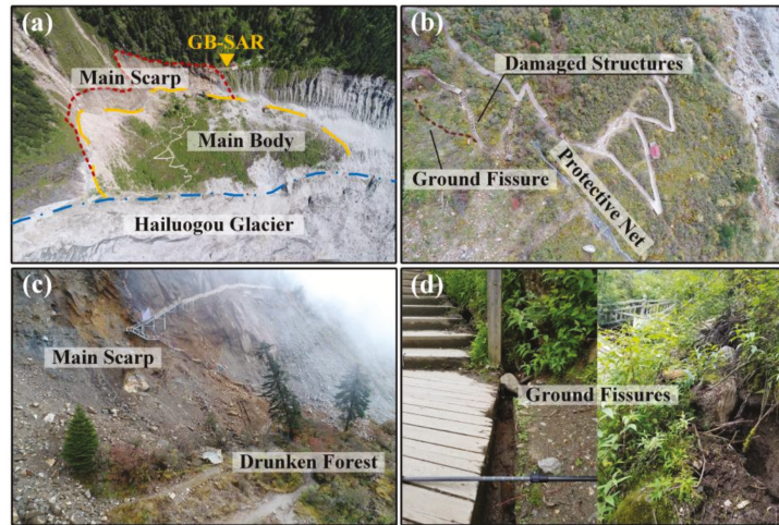
Figure 6. LGJT landslide on the Hailuogou Glacier. (a) Overview of LGJT landslide. The main scarp that formed by the separation of the rear edge of the landslide's main body from the mountain mass is very prominent. The front edge of the landslide body is tangent to the Hailuogou Glacier and local collapse is notable. (b) Detailed landslide surface structures can be observed such as partially damaged footpaths, the rockfall protection net, and ground fissures. (c) Details of the main scarp and rear edge of the main body. The altitude difference of the main scarp is >50 m, which causes the trees below to seriously incline and appearance of the unique phenomenon of a drunken forest in the landslide movement. (d) Ground fissures on the surface of the landslide; the fissure width generally ranges from 15 to 30 cm.
