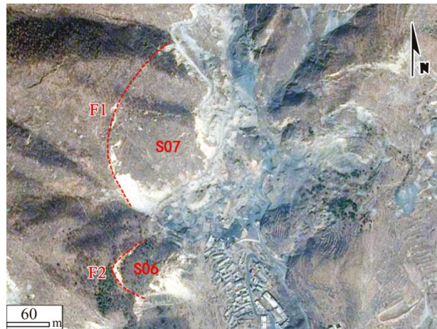
----- Rear part fissures of landslide
