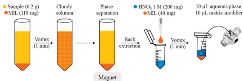
Figure 3. Scheme of the analytical procedure for Cd quantification. Reproduced with permission from [43]. Copyright Elsevier, 2020.
