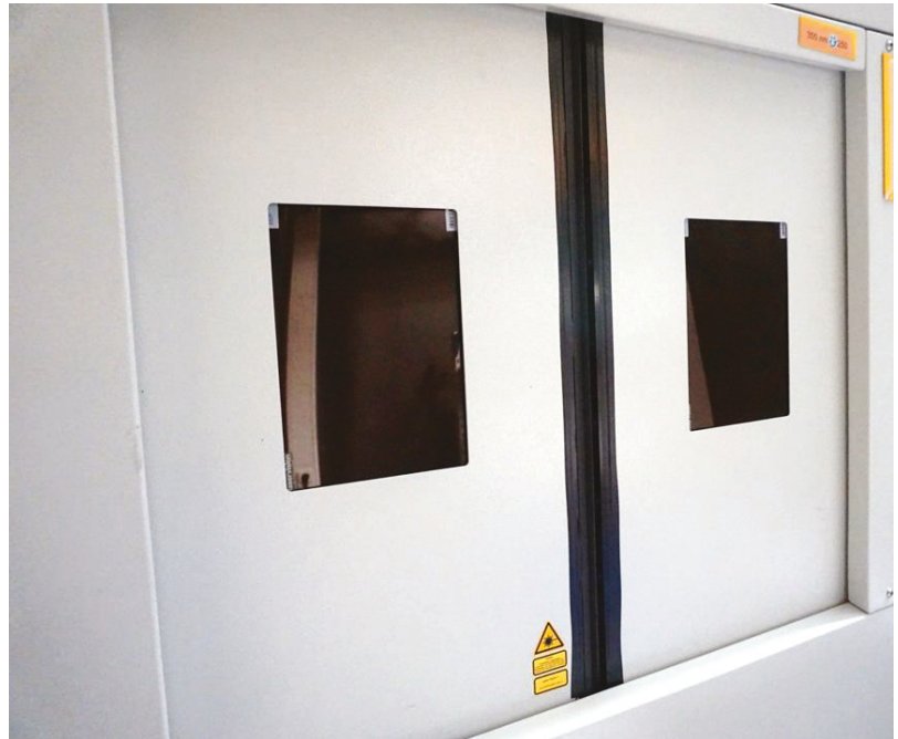
Figure 9. Photograph of the protection housing doors of the second experimental setup. The laser used in the system is a Coherent HR50 USP-laser with an average power of 35 W. The housing is made of 2 mm thick steel, and the windows are made of PMMA covered with a thin sheet of aluminum. Between the two doors there is a narrow area where, in the closed position, only rubber material lips join without any additional steel or aluminum layers.
