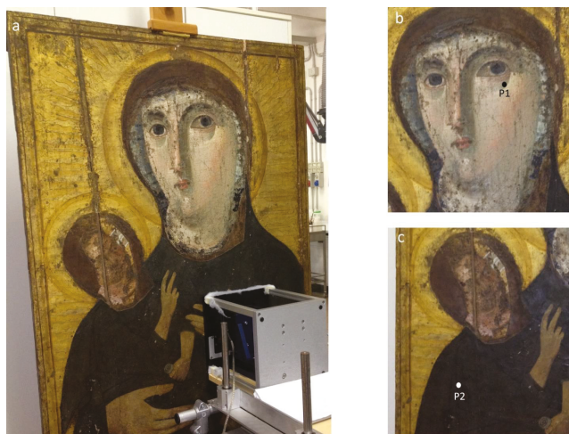
Figure 11. (a) Single-sided NMR collecting a stratigraphy of the Madonna Hodigitria icon. (b,c) Details of two regions of the icon measured by NMR. Adapted from [19].
