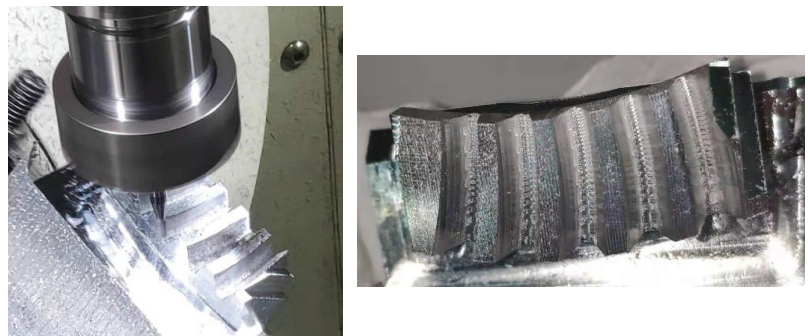
Figure 12. Five-axis flank milling of SBG.
