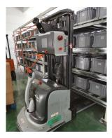
Figure 1. Forklift AGV.
