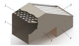
**Figure 2.** A separator with arc-shaped elements (a cross-sectional view): (1) the inlet for the gas contaminated by the catalyst; (2) rows of arc-shaped elements; (3) the body; (4) the hopper; and (5) the outlet for purified gas.
