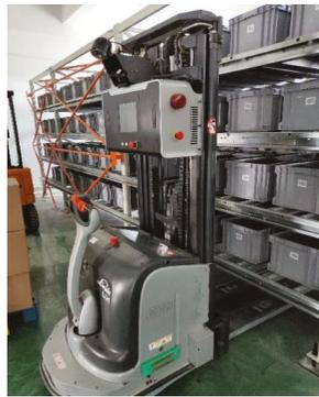
**Figure 1.** Forklift AGV.
