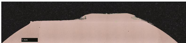
Figure 15. Plateau forming due to axial material flow of lower electrode of MC02–TS02 after 822 spot welds in cross-section [11].
