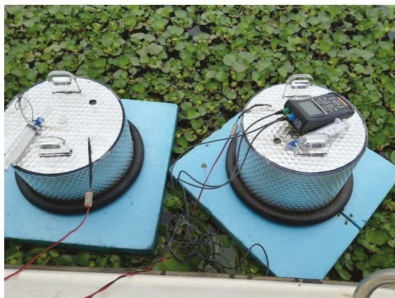
Figure 2. The measuring chambers at the invasive water hyacinth site (ECs) of Hong Lake.
