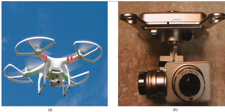
Figure 1. Details of the DJI Phantom 2 Vision+. (a) General image of the quadcopter; and (b) the details of the camera.
