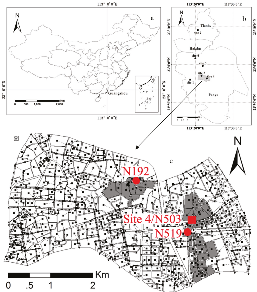
Figure 1. The locations of Guangzhou (a); meteorological sites (b); and the three selected nodes and their catchment area/ modeling areas by SWMM in Panyu District (c). Street flooding water depth is recorded near Site 4/Node 503 by a wireless electronic water depth meter.
