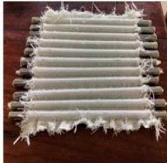
(b) Insertion of rods in hollow knitted structures
