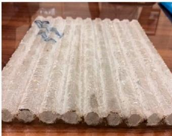
(d) Recycled cotton fiber based hollow composite
