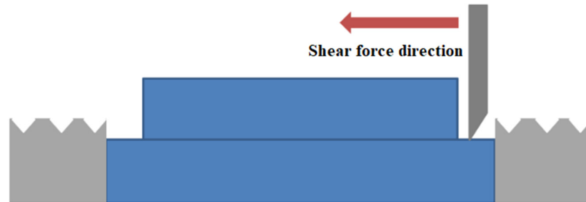
Figure 8. Schematic diagram of shear force test.
