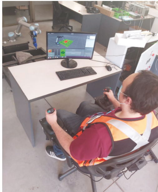
Figure 17. User operating the UR5 arm, using the haptic controls (installed on a chair), and the user interface.
