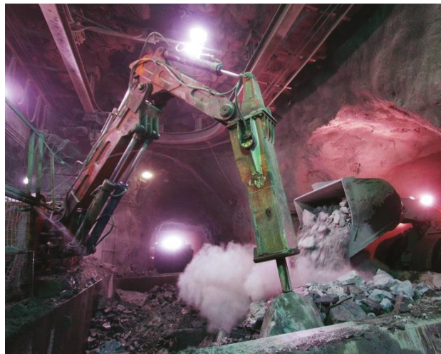
Figure 2. Real impact hammer in operation, while material is dumped onto the grizzly.
