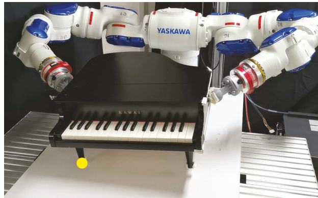
Figure 1. A dual-arm robot manipulates a piano by pivoting on the object’s vertex (marked by a yellow dot).
