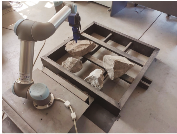
Figure 15. Experimental operation of the rock breaker set-up.
