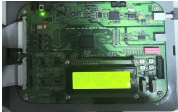
Figure 9. Cyclone-IV EP4CE30F484 FPGA controller.
