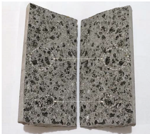
Figure 16. Splitting tensile failure.
