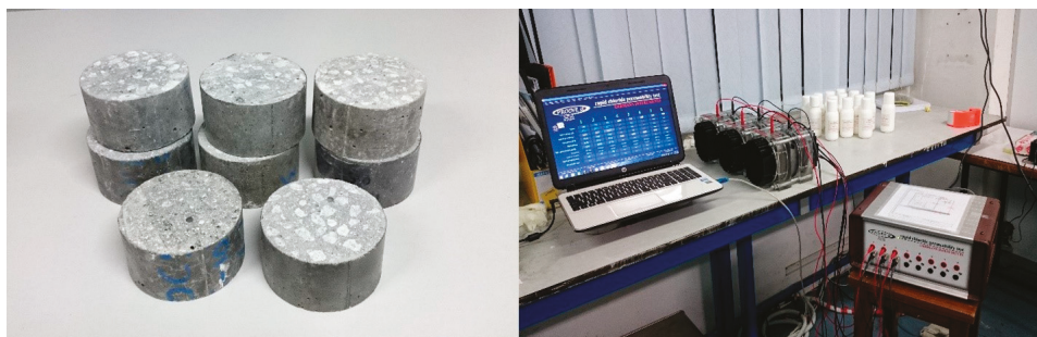
Figure 29. Concrete specimens and test set up (ASTM C1202).
