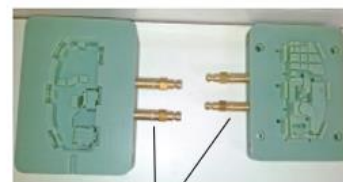
Cooling system -External
