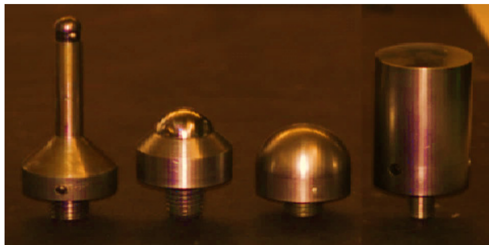
Figure 3. Indentation, different sizes of punch are used, which are hemispherical punches of diameters 12 mm, 28 mm, and 44 mm, and a flat cylindrical punch of 25 mm.
