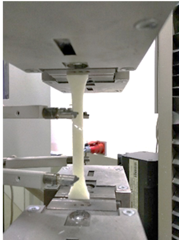
Figure 5. Tensile test according to ISO 527 on machined out standard test specimens of the PP/GF30 injection molded short fiber-reinforced thermoplastic composite.
