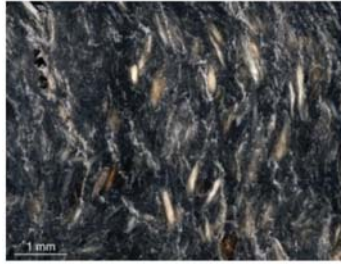
Figure 2. Microscopic structure of wood–plastic composite material—cracks at the interfaces (Nikon Eclipse 80i, Tokyo, Japan) [55].
