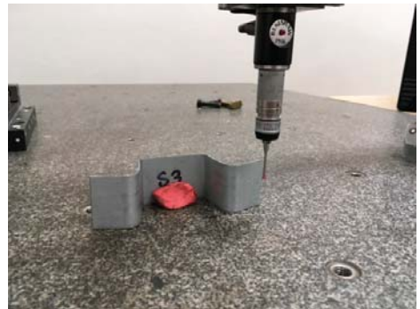
Figure 12. Determination of the specimen actual shape (device SOMET XZY 464).
