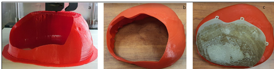
Figure 7. (a) 3D printed skull model of the ABS material with supports, (b) ABS skull model after the removal of the supports, and (c) the rehearsal and fitting evaluation of the PEEK cranial implant on the ABS skull model.
