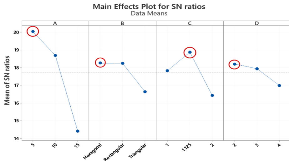
Figure 5. Main effect plot circularity. A, B, C, and D represent the Thickness, Infill Pattern, Layer height, and Wall Layer, respectively.
