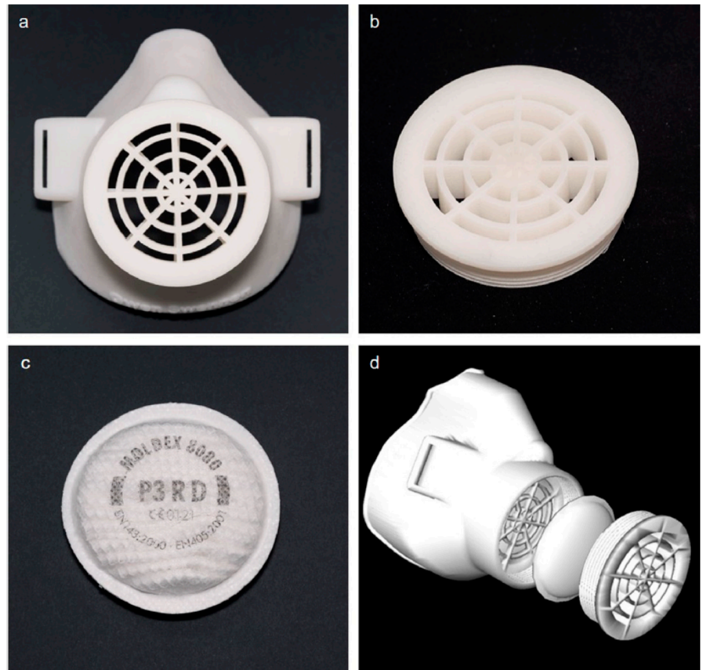
Figure 9. Typical representation of the 3D-printed face mask: (a) reusable 3D printed face mask, (b) filter membrane support, (c) polypropylene (PP) nonwoven meltblown particle filter, (d) 3D image of the prototype [52].
