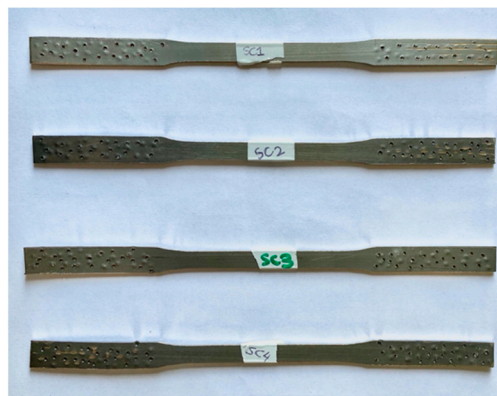
Figure 2. Dog-bone specimens used for the fatigue tests.
