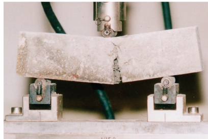
Figure 3. Measurement of the bending strength via three-point bending.
