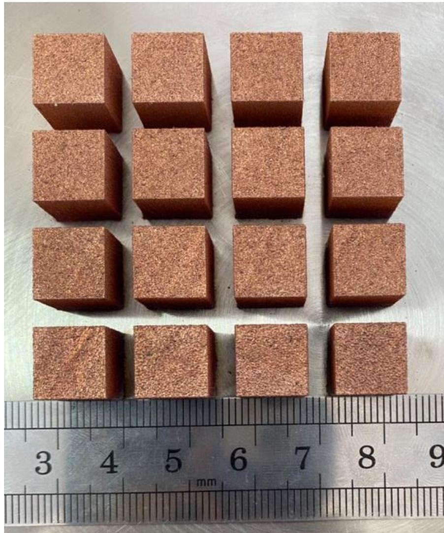
**Figure 3.** CuCrZr samples fabricated by SLM.
