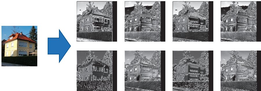
Figure 16. Effect of the Gabor filters on an input house image: The top row images are produced by Gabor filters with a kernel size 5, sigma 2, and theta having the following respective values: 0, 45, 90 and 135 degrees (from left to right). The bottom row images are produced by Gabor filters with kernel size 5, sigma 5, and theta having the following respective values: 0, 45, 90 and 135 degrees (from left to right). (Source of input image: own image).
