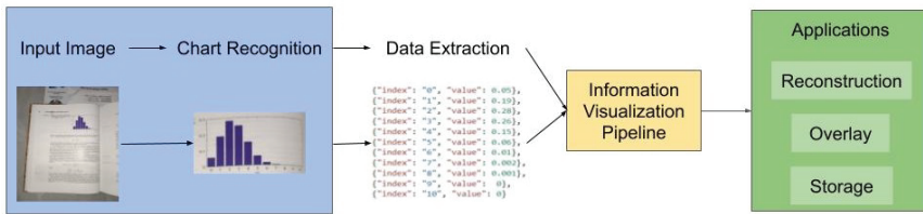
Figure 2. Automatic main process of chart recognition, from the input image to applications. The main process can transform a static environment in a rich user interface for manipulation of data. The information visualization pipeline is environment free, allowing the applications to be used in many environments. This is only possible when the initial step cleans the chart and gives information (blue area).
