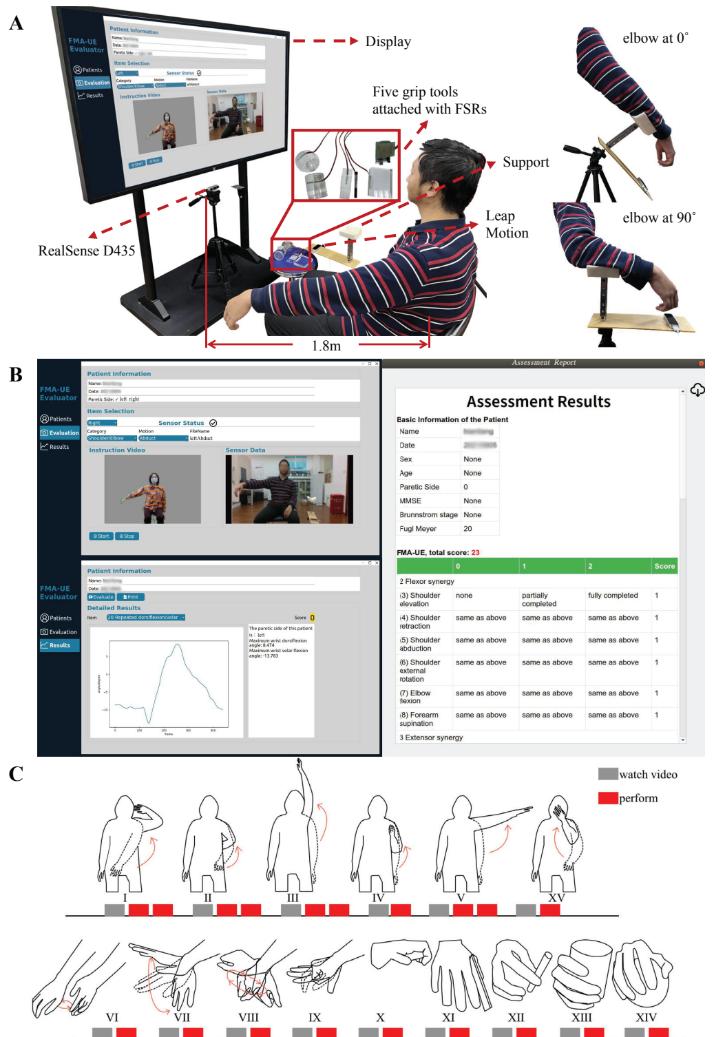
Figure 1. (A) The hardware setup and scene of the experiment. On the right are the two initial positions for the Wrist/Hand part. (B) The graphical user interface (GUI) of the assessment system. (C) The experimental protocol.
