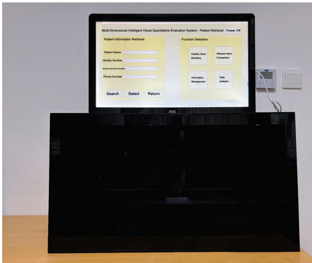
Figure 4. Hardware platform prototype of MDIVQAS.
