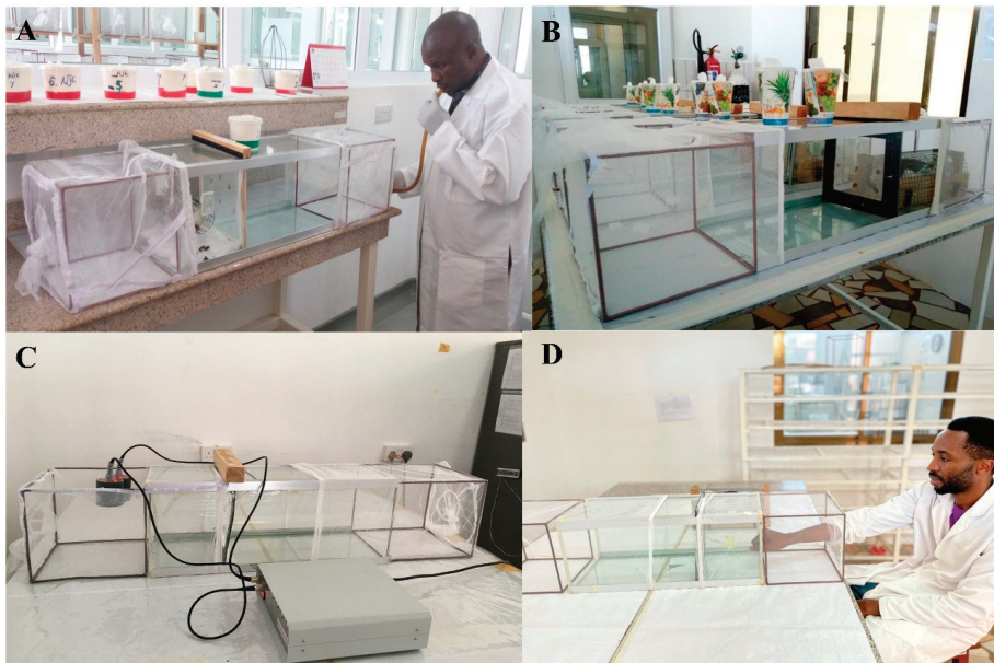
Figure 1. WHO tunnels for comparison of baits: (A) Conduct of standard WHO Tunnel with the bait chamber to the left of the picture and mosquitoes being placed into the longer end of the chamber; (B) Rabbit—in Experiments 1–4; (C) Hemotek ® membrane—in Experiment 1 and 4; and (D) Human arm—in Experiment 1.
