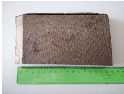
Figure 1. Illustrative cross-section from VVER-440 RPV (Original not-irradiated piece from VVER-440 V-213 RPV—Greifswald Unit 7).
