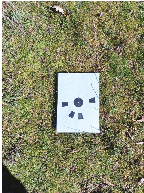
Figure 2. Printed GCP pattern, distributed throughout the survey area during UAV campaigns.
