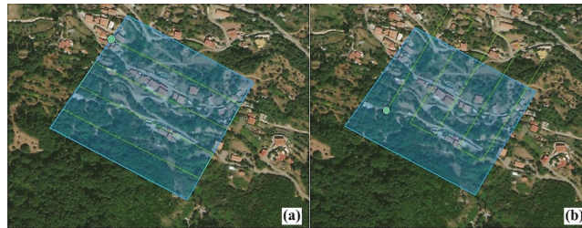
Figure 5. UAV acquisitions over the landslide of Messarista. (a) Nadir-viewing acquisition trajectory; (b) Oblique-viewing acquisition trajectory.
