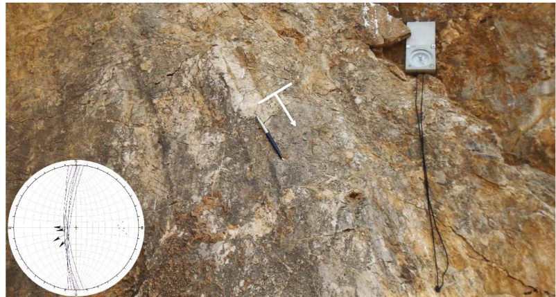
Figure 5. Fault plane of a Kastelli fault segment measured at 74/263, on which striations measured at 61/220 were found (parallel to the pen), confirming the oblique normal movement with left-lateral component. Measurements at several places are plotted in the inset diagram.
