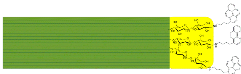
Figure 1. A cellulose nanorod, represented according to the model proposed in [32], with 1-pyrenyl units attached to the reducing ends (highlighted in yellow) by reductive amination.
