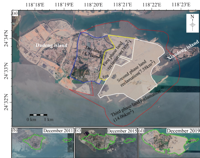
Figure 2. Optical images of the XXIA, Dadeng Island, and Xiaodeng Island: (a) illustration of the three phases of land reclamation. The yellow, white, and red lines are the boundaries of the reclaimed land in the first, second, and third phases, respectively. The blue line represents the dry land of Dadeng Island; (b–d) optical images of the study area acquired in December 2011, December 2015, and December 2019, respectively. The green lines delineate the boundaries of Dadeng Island and Xiaodeng Island.
