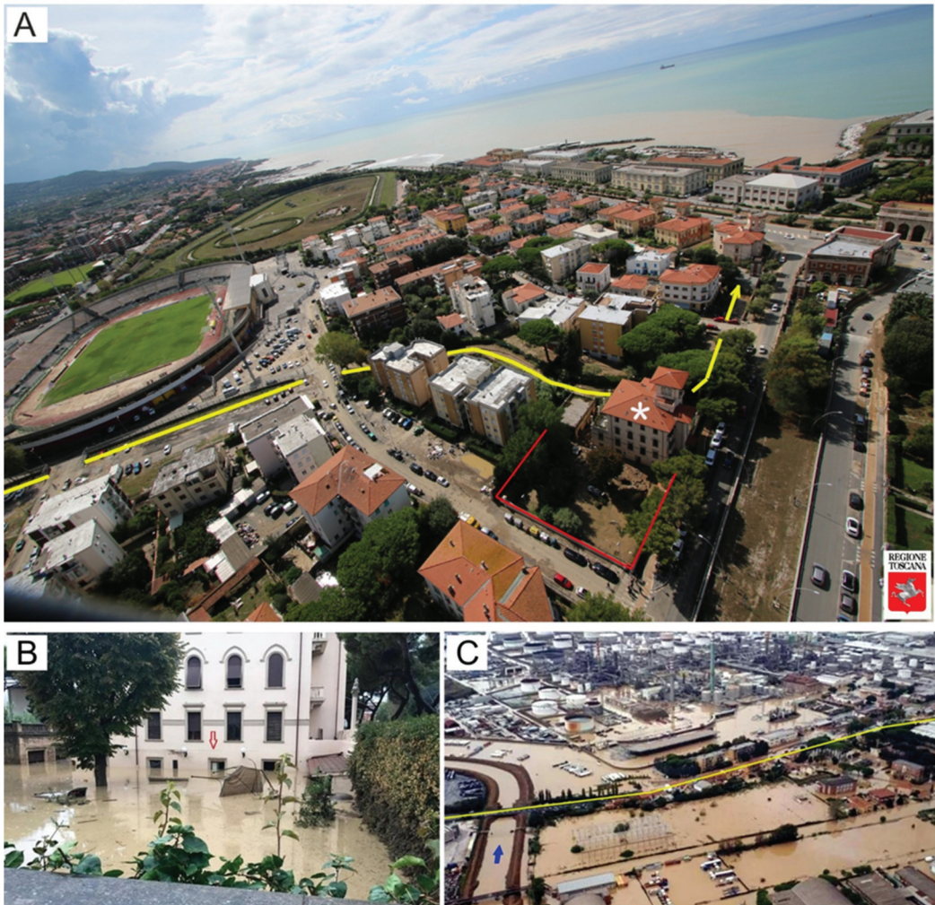
Figure 10. Livorno. (A) aerial photograph of the Ardenza Stadium district. In the foreground is the house where the four victims drowned (white asterisk). The yellow line highlights the culverted streambed of the Rio Maggiore: its flood waters were the cause of the rapid flooding of the courtyard (evidenced by red lines) and of the ground-floor flat [58]. (B) Livorno: the house where four people from the same family drowned (courtesy of Il Tirreno). Their ground-floor flat is located at the end of a large courtyard, below street level on Rodocanacchi Street (area of the Ardenza football stadium). The red arrow indicates the level reached by the floodwaters in a few minutes. (C) Livorno: the Stagno district that was largely flooded by the Rio Ugione floodwaters with the Via Aurelia (yellow line) and the refineries in the background [58].
