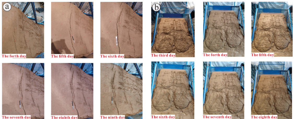
Figure 14. Deformation and failure process of fill slope under rainfall. (a) Crack development process near slope shoulder and (b) shallow sliding process.
