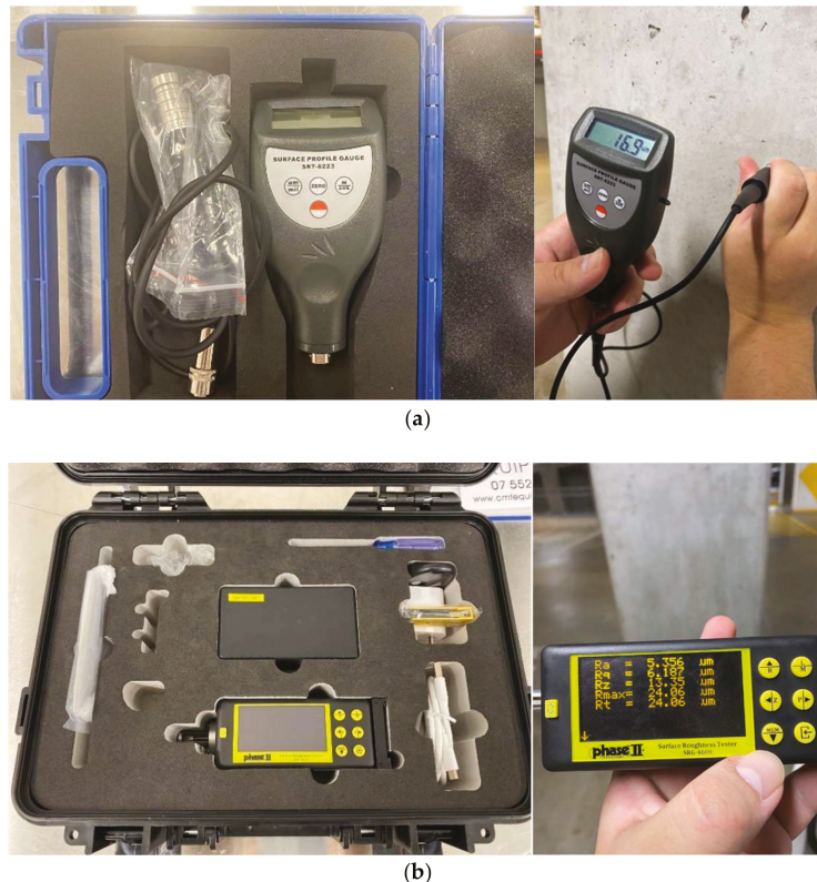
Figure 9. Portable surface roughness gauge: (a) surface profile gauge (large range and low resolution); (b) surface roughness gauge (low range and high resolution).
