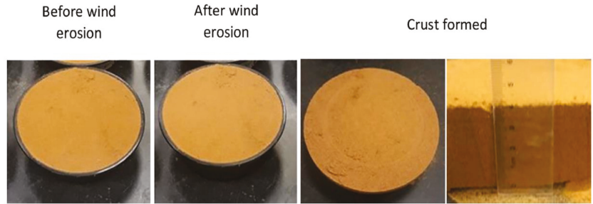
Figure 8. Crust formation of sand treated by sodium alginate biopolymer [145].
