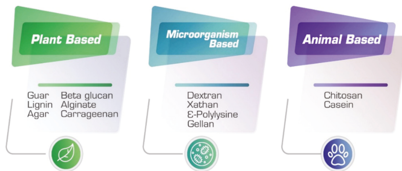
Figure 1. Common biopolymers used for soil improvement based on their source of production.
